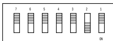
Figure 2-1, Switch S1 (Set to Logical Address 2)
