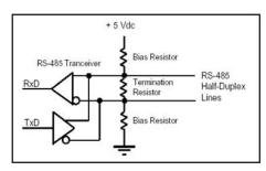
The figure shows how the terminating and bias resistors are used in a typical half-duplex circuit. If the serial channel is being used for RS-485 data transmission, an internal set of termination and bias resistors can be switched on the Tx/Rx signal pair. For RS-422 data transmission, the resistors can be switched on the Tx signal line. Standard values are 150 ohms for the load resistor and 2.2 k ohm for the pullup and pulldown bias resistors.
