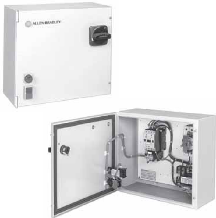
IP66 (Type 3/4/12) Enclosure With Optional Start-Stop Push Button, Pilot Light and Control Circuit Transformer
