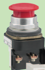
Copper terminals/spanner and silver nickel contacts to carry higher currents
