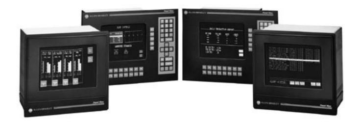
PanelView™ 1200 Operator Terminals are the original PanelView terminals designed to replace traditional hard-wired panel devices ①, such as (push buttons, bar graphs, digital readouts, and message displays) with CRT screens that are simple to configure. Use PanelView 1200 terminals in control panel applications that connect to Allen-Bradley PLC controllers over a Universal Remote I/O link.
