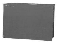
As members of the Allen-Bradley family of high-performance open systems, 6180 Industrial Computers can be ordered with pre-installed software products including popular operating systems and MMI and control software.
