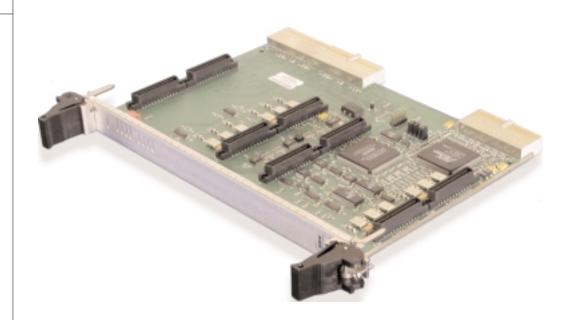
**SBS' CPCI-200B-BP IndustryPack carrier board** provides four IndustryPack slots on a 6U CompactPCI card. The CPCI-200B-BP provides IndustryPack I/O via the CompactPCI J4 and J5 connectors. Rear panel transition modules, BIO-3 and BIO-4, are available from SBS.
