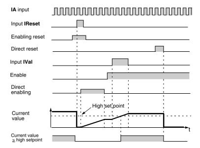
The time diagram below shows a triggered reset on the rising edge of **IReset** input, a direct (software) reset and an automatic reset when crossing the high setpoint.
