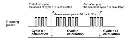
The sampling period must be chosen according to the required precision and the low limit of the speed (frequency) of the signal to be measured. This is done using the following formula:
