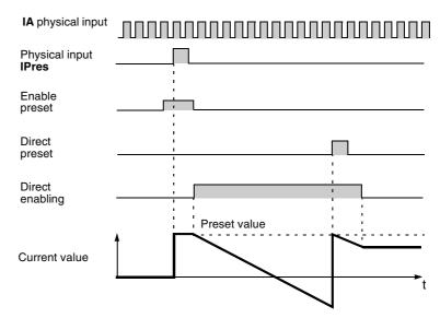
The time diagram below shows a preset triggered by **IPres**, a direct preset, and an automatic preset when crossing the zero value.
