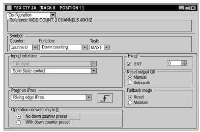
The C sensor (for counting the objects) is mated with the 0 channel.
