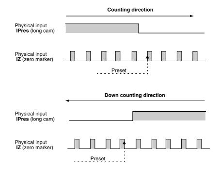
**Note:** preset is taken into account on the first rising edge of the **IZ** revolution marker input, which follows the change of **Ipres** input to status 0, both in the counting and the down counting directions and software enabling.
