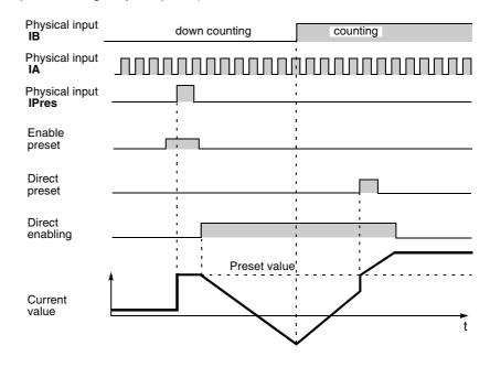
Preset on IPres edge combined with counting direction The figure below shows an example of preset on the rising edge of **IPres** in up counting (+ direction), and on the falling edge of **IPres** in down counting (- direction). The reverse case is similar.
