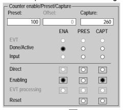
Clicking on this button sets the associated bit to 1. The button and possibly the LED above light up (switch to a color).
