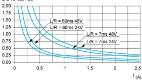
DC13switching electromagnets, L/R ≤ 2 x (Ue x le) in ms, Ue: rated operational voltage, le: rated operational current (with a protective diode on the load, DC12 curves must be used with a coefficient of 0.9 applied to the number in millions of operating cycles)
