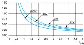
AC15control of electromagnetic loads > 72 VA, make:  $\cos \varphi$  = 0.7, break:  $\cos \varphi$  = 0.4.
