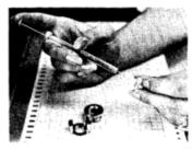
For handling small liquid samples, the Wilks Sealed Ultra-Micro Cells offer the spectroscopist a wide choice of materials and volumes. The cell is constructed of two 13 mm discs cemented to a spacer and can provide sample volumes between 0.17 and 2.28 µl.
