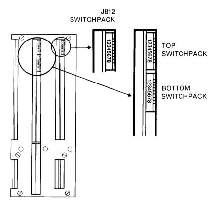
All switch settings are referred to as "to the left", "L", or "to the right", "R", left being off and right being on.
