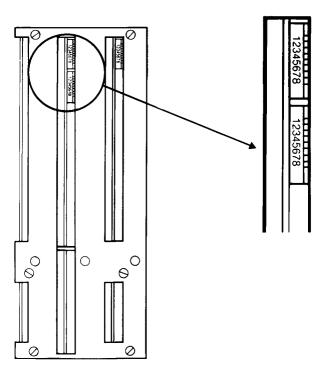
By selecting the size of the housings, the maximum number of housings allowed in the subsystem is determined since there is a maximum configuration of 32 slots. This configuration is obtained by using all the available slots starting with rack one, slot four and numbering the slots 1 to 16 then 1 to 16 again. One set of 16 can be used for input only and
