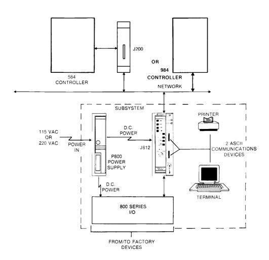
As shown in Figures 2-1 and 2-2, the J810/J812 is the adapting interface between the controller and the I/O. The 584 or 984 PC communicates with remotely located I/O drops through a coaxial cable network. The subsystem address and supported I/O configuration are identified by switch settings in the J810/J812.
