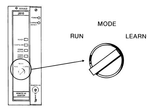
When in LEARN mode, the J810/J812 writes zeros to all output modules. Equipment which is sensitive to zero data should be disconnected prior to switching to LEARN mode.
