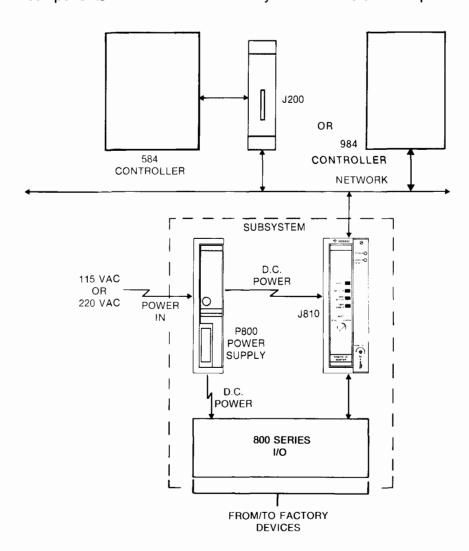
The J812 Adapter Module has the same functions as the J810 and also supports two ASCII communication ports. This allows terminals, printers, and other peripherals to be added to the system. Figure 2-2 shows the J812 subsystem or remote I/O drop components.
