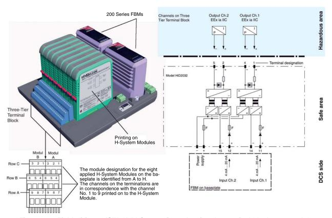
Figure 4-1. Field wiring to ISTA-\*BP\* Connections showing the terminal blocks per module
