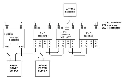
Figure 1-8. Diagram of HART Mux Installation
