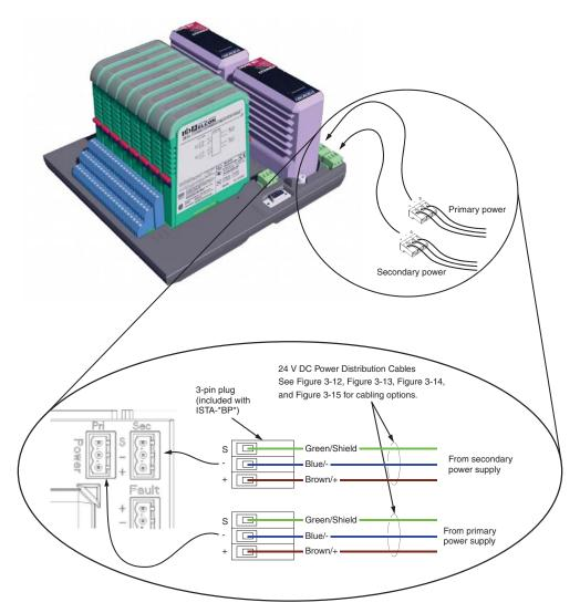
Figure 3-12. Power Supply Cable Connections at ISTA-\*BP\*
