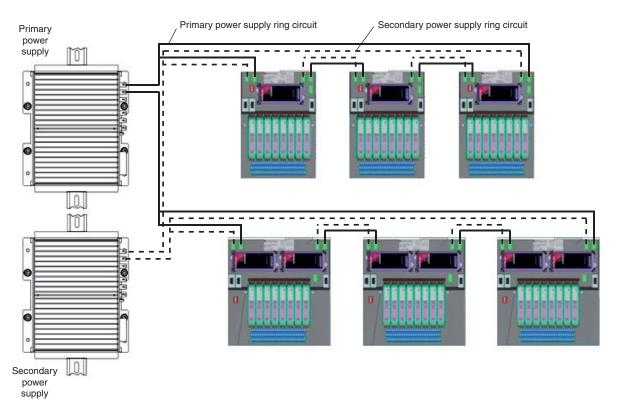
Figure 3-11. FPS400-24 Power Supply Wiring
