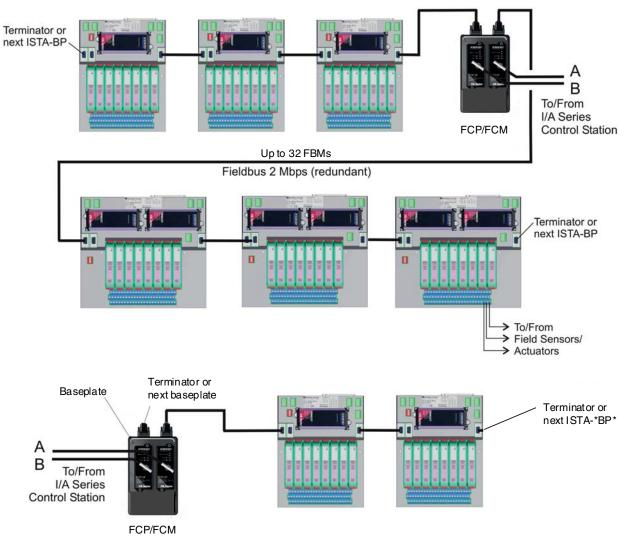
Figure 1-1. Layout of an ISTA-\*BP\* System
