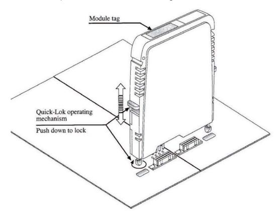
Figure 3-4. Mounting of H-System Modules on ISTA-\*BP\*
