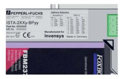
Figure 3-15. Addressing a Non-Redundant, Dual or Redundant ISTA-\*BP\*
