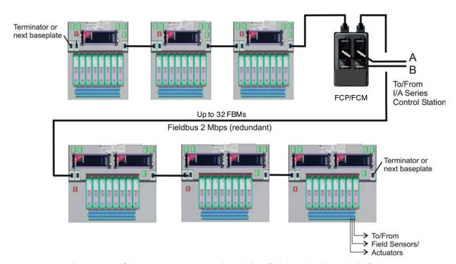
Figure 1-3. ISTA-\*BP\* Interconnection Using Shielded Twisted-Pair Cable
