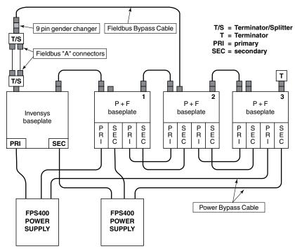
Figure 1-5. Bypass Connection First Baseplate
