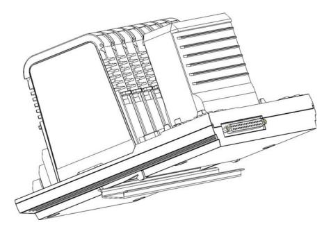
Figure 3-2. Mounting of ISTA-\*BP\* on DIN Rail
