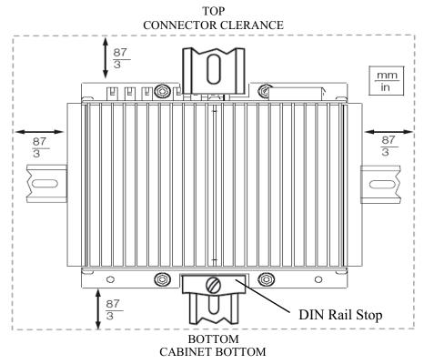
Figure 3-7. Foxboro Power Supply FPS400-24 Clearance Requirements
