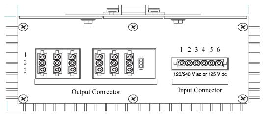
Figure 3-9. Input and Output Power Connector from FPS400-24 to Baseplate Connector for Version P0922YU
