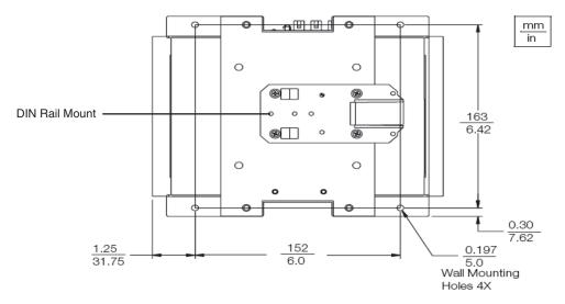
Figure 3-8. Foxboro Power Supply FPS400-24 Wall Mount Bracket Screw Hole Dimensions
