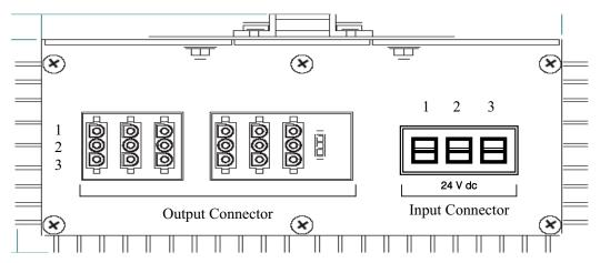
Figure 3-10. Input and Output Power Connector from FPS400-24 to Baseplate Connector for Version P0922YC
