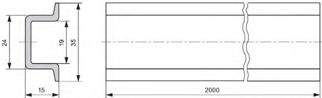
Figure C-4 Dimensional drawing of the 2000 mm standard rail
