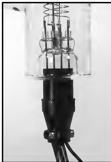
Figure 1-9. O100C1 4-pin connector safely attached to the base of the glass-tubulated gauge.
