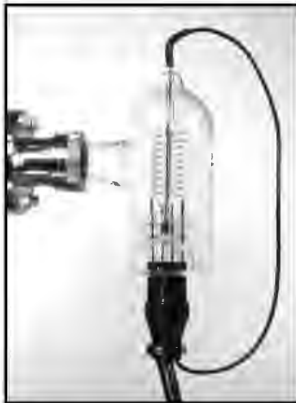
Figure 1-11. Picture of properly and safely connected glass-tubulated ionization gauge.
