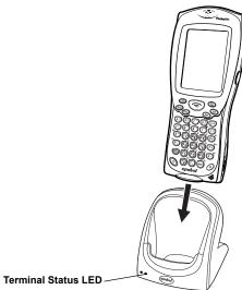
3. The Terminal Status LED turns red (may take up to one minute) to indicate charging, then turns off when the battery is fully charged. The terminal's battery is fully charged after approximately 2 1/2 hours.
