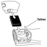
Replace the battery cover, pressing down firmly along the top edge while sliding the latches down into the locked position.
