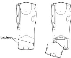
2. Insert the lithium-ion battery in the battery compartment with the battery tether positioned properly (as shown below), making sure the battery snaps into place.
