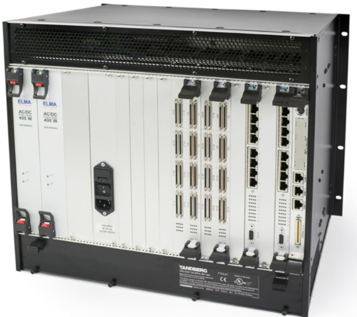
Figure 8-12. PRI E1/T1 and V.35 interface cards, MPS 800
