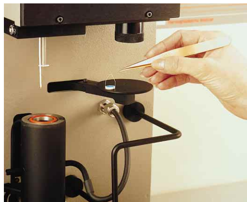
Figure 4 Placing sample pan on platform
