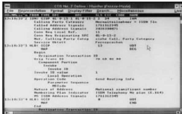
Fig. 1 SCCP-HLR data exchange in the GSM.
