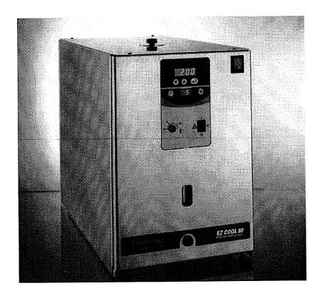
This device contains safety elements according to category NFL making it suitable for unattended continuous operation with non-combustible substances as bath liquid (water or water with antifreeze).
