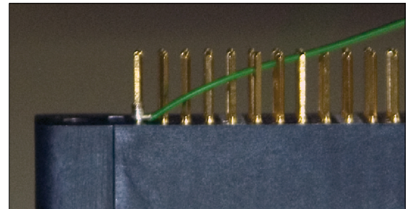
Figure B. Completed wrapped wire.
