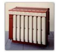
The Target® ARS is a rack-based, modular system that can be customized for each application with additional Axis Modules and Digital/Analog I/O Modules. Link two Target® racks to create a powerful system that provides up to 8 axes of control, more motor power, and up to 512 digital I/O.
