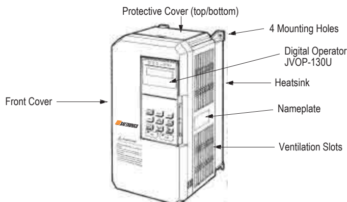
Figure 3 Parts Identification - Model CIMR-VG5U43P7
