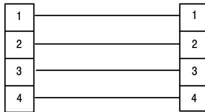
Figure 2.11 Recommended Wiring for Backup Cable Linking a KP3 to an S4A, S5, or MX Module
