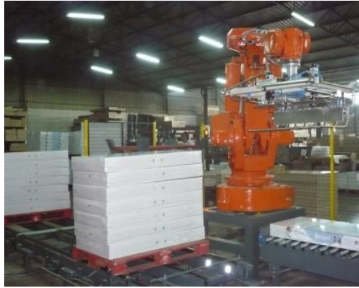
This 150kg IRB6000 was installed by our customer in Portugal
