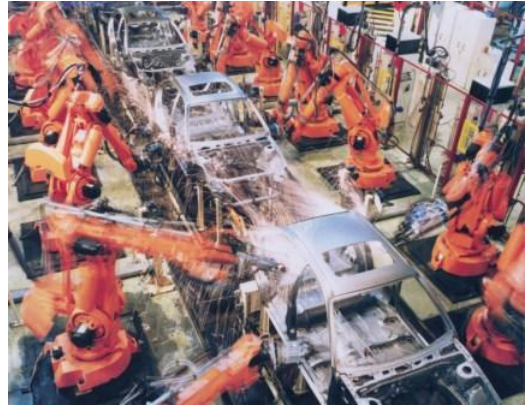
IRB 6000 robots spot welding in an automotive plant
