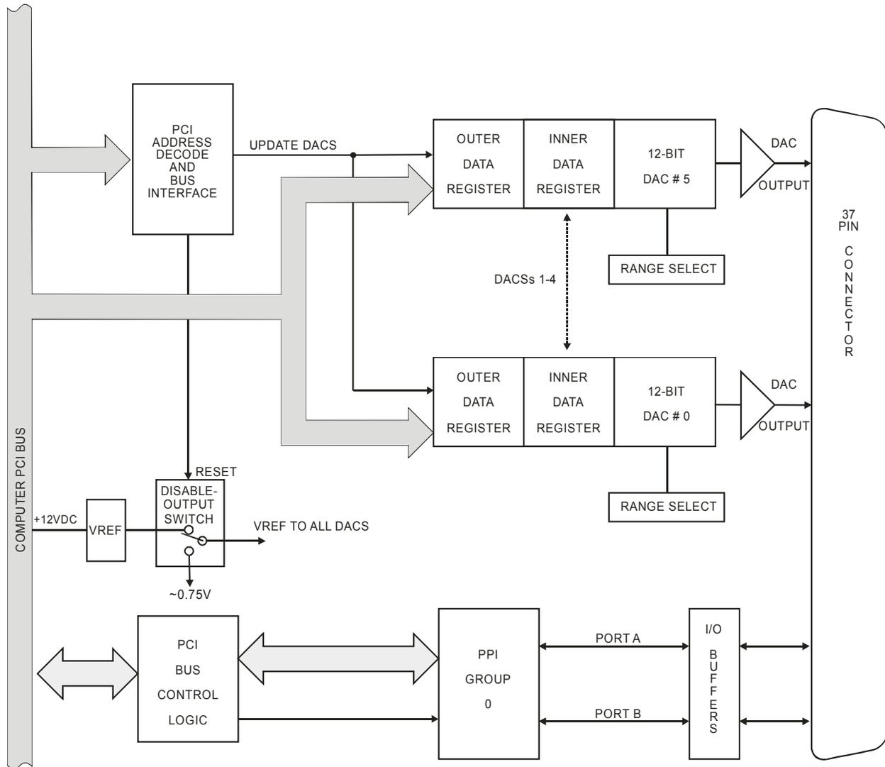
Figure 1-1: Block Diagram
