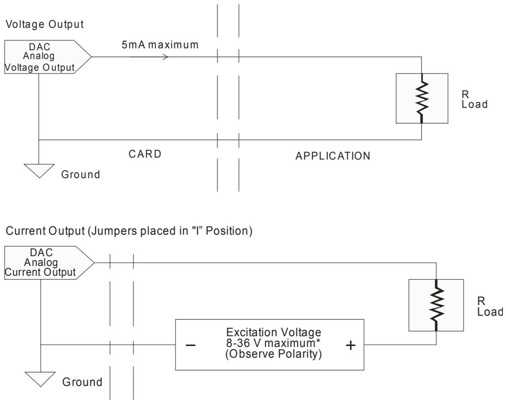
**Figure 3-2: Field Wiring**
