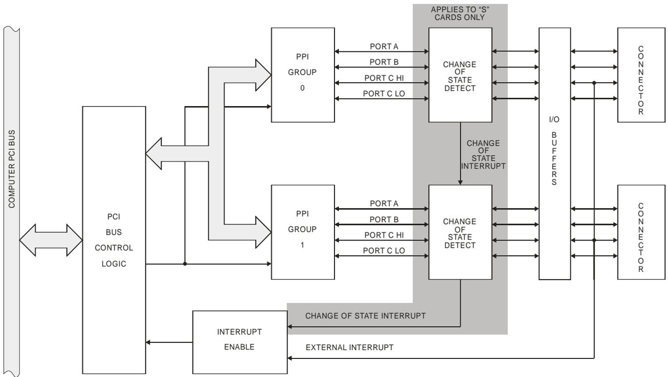
**Figure 1-1: Block Diagram**
