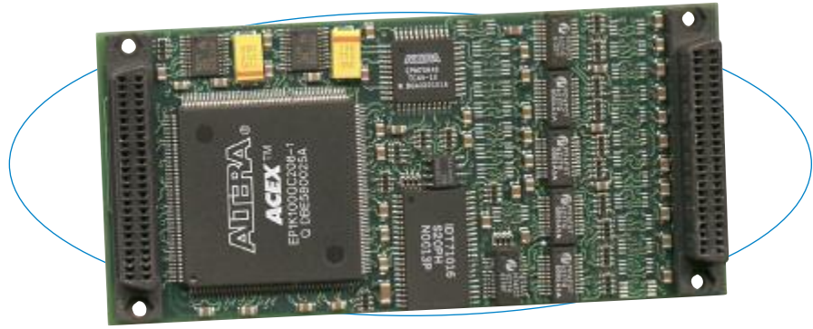
These modules support adaptive computing applications with an FPGA running custom programs to control system communication.
