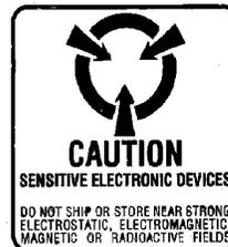
This board is physically protected with packing material and electrically protected with an anti static bag during shipment. However, it is recommended that the board be visually inspected for evidence of mishandling prior to applying power.
