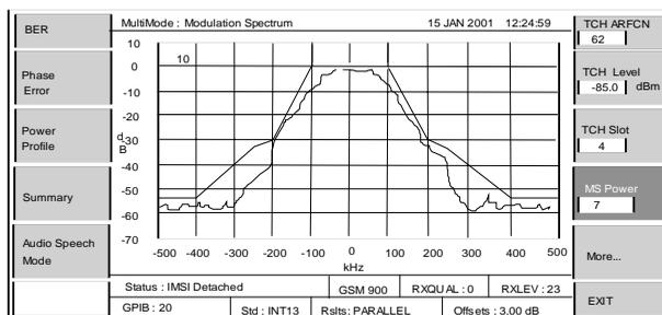
*Real-time displays for displays for simple with superimposed limit mask*
