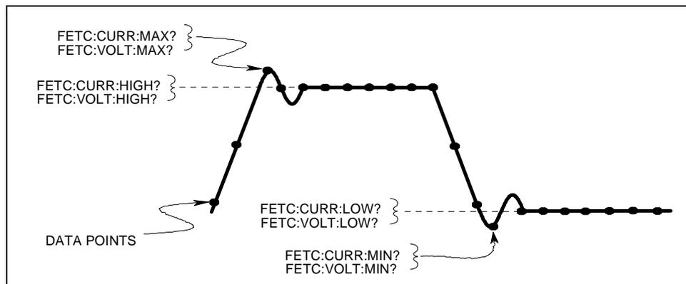
**Figure 3-4. Measurement Commands Used to Return Pulse Data**
