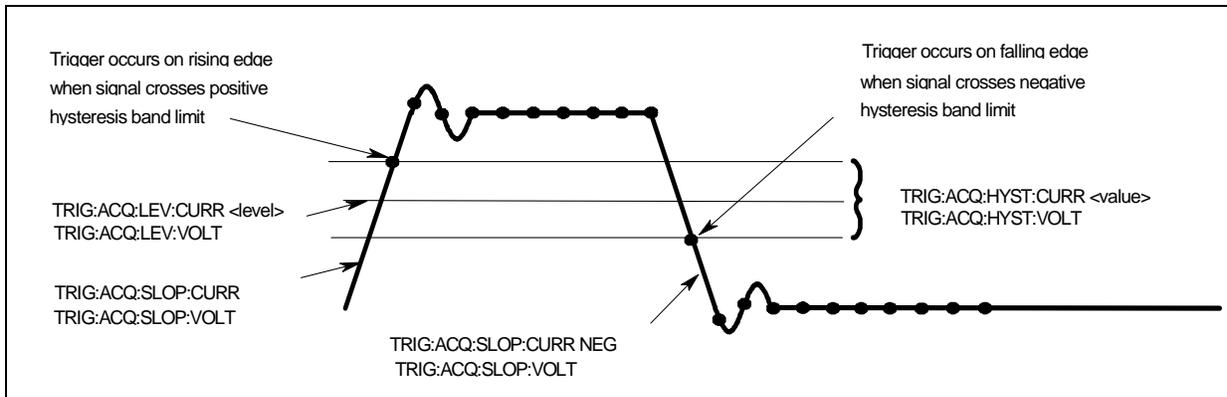
**Figure 3-3. Trigger Commands Used to Measure Output Pulses**
