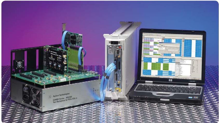
Figure 1. E2960B Series PCI Express Analyzers
