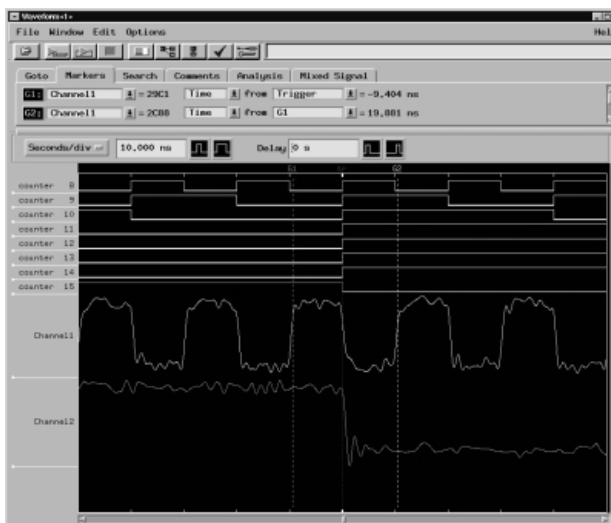
Figure 5.25. Infiniium oscilloscope waveforms are displayed in the 16700 logic analyzer waveform display window along with logic analyzer timing waveforms, accurately time-correlated.
