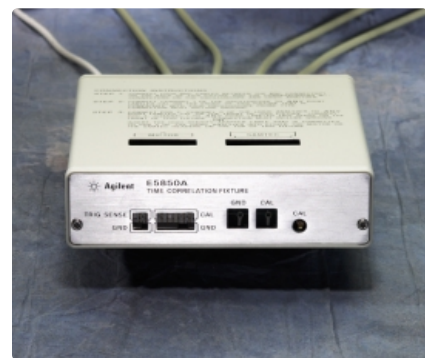
Figure 5.26. E5850A time correlation fixture.
