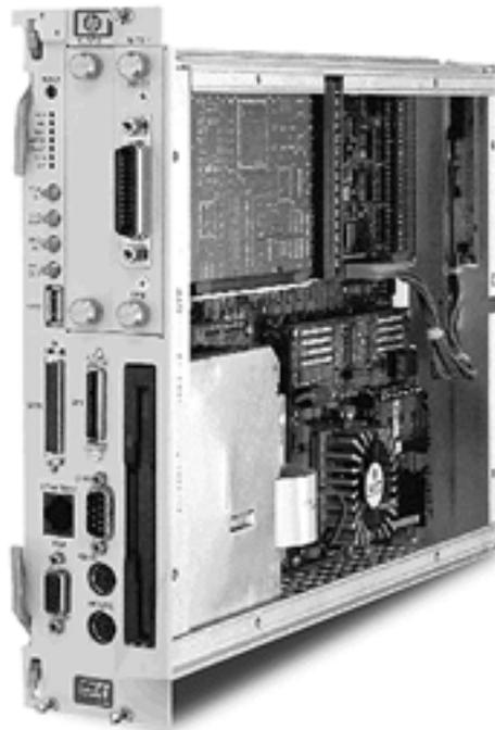
**Figure 1-1. The HP VXI Pentium Controller**
