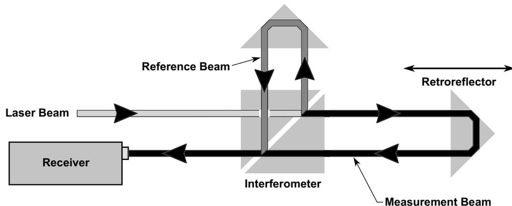
**Figure 4-6. Optimum alignment**
