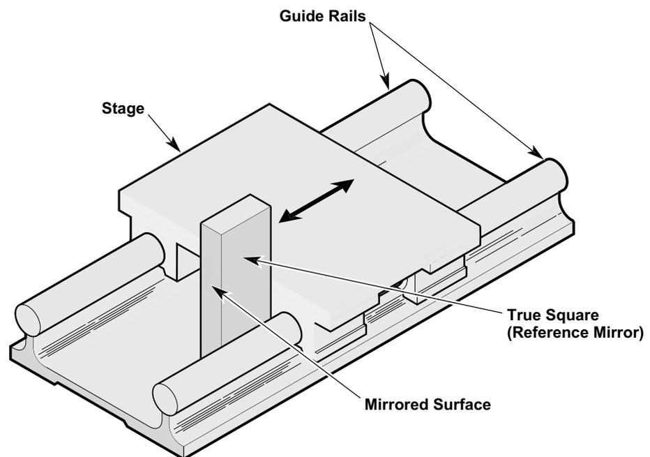
**Figure 4-9. Using reference surfaces to align mirror**
