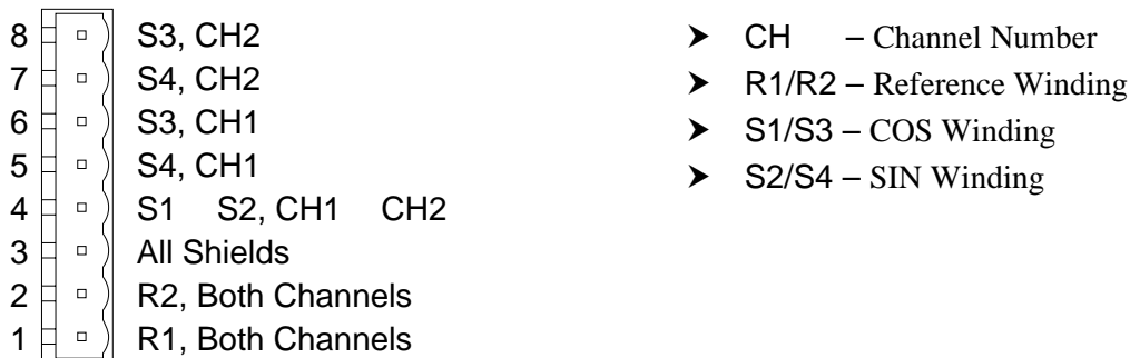
Figure 2.20 Transducer Input Connector
