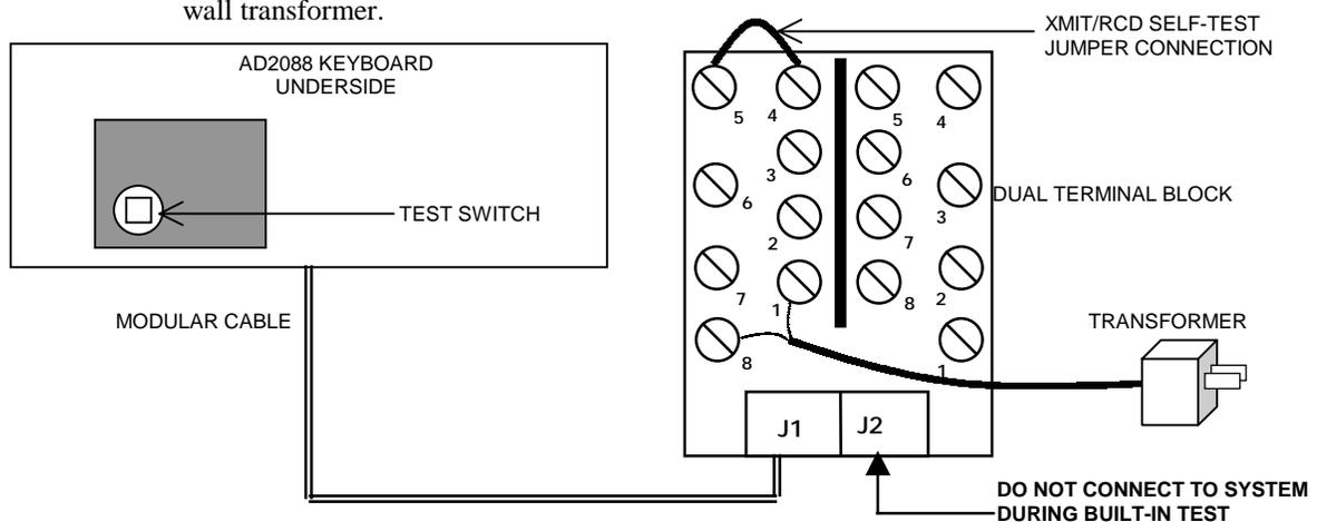
Each test is performed in sequence. Press the test switch button to advance to the next test procedure. To quit the test sequence, unplug and then re-plug the wall transformer.
