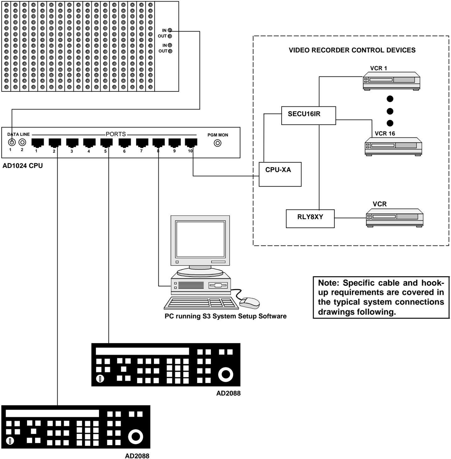
**Note:** Specific cable and hook-up requirements are covered in the typical system connections drawings following.
