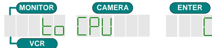
5. The number in the ENTER display indicates the percentage of macros successfully transferred to the keyboard. The number starts at 0 and increases in increments of 10, up to 100 percent. With the keyboard set to 9600 baud and connected directly to the CPU, the transfer will take up to three minutes. With the keyboard set at 1200 baud and connected through a Port
