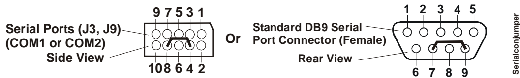
Figure 3-2. Hot Cable Jumper
