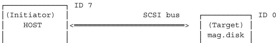
A SCSI system may be as simple as a single computer with SCSI host adapter connected by cable to a single SCSI Target device, such as a disk drive.
