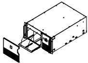
2. Unhook the side of the cover from the chassis and lift it away to expose the battery door.
