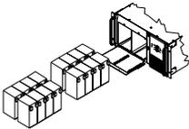
5. Hold the battery pack so that the leads are on the right hand side and the battery terminals are at the top edge of the battery. Slide the battery pack into the UPS. Press the gray connector into the plug at the right-hand side of the battery compartment. Tuck the white cord (that serves as a handle for the connector) neatly to the side.
