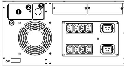
3. Slide the wire input plate ❸ to the left to remove it. This will expose the input wiring terminal.
