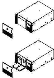
1. Remove the front bezel by grasping the finger clips on the side of the bezel and carefully loosening the four (4) snaps.
