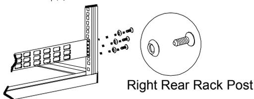
1. Determine where in the rack you will mount the UPS. The SU5000 requires a space of 5U. Some racks have tick marks to indicate the U-spaces.
