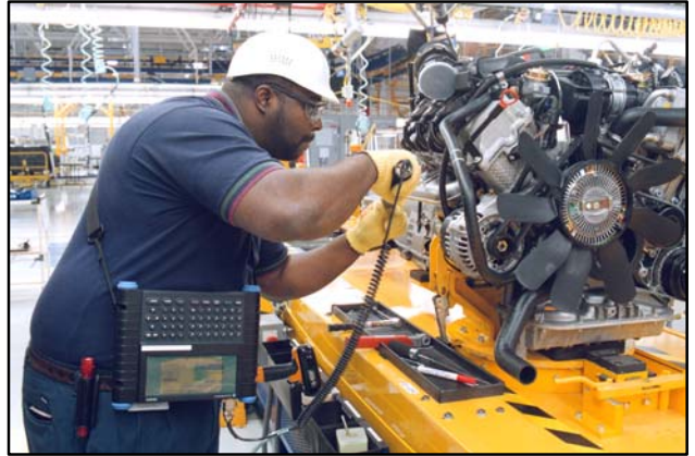
The 3053 is ideally suited for roving torque audits.
