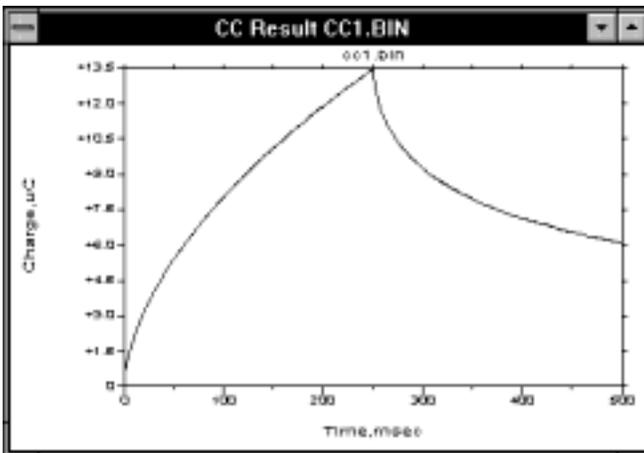
**Figure 10-7.** Chronocoulogram (charge-time) response for double-potential-step CC.
