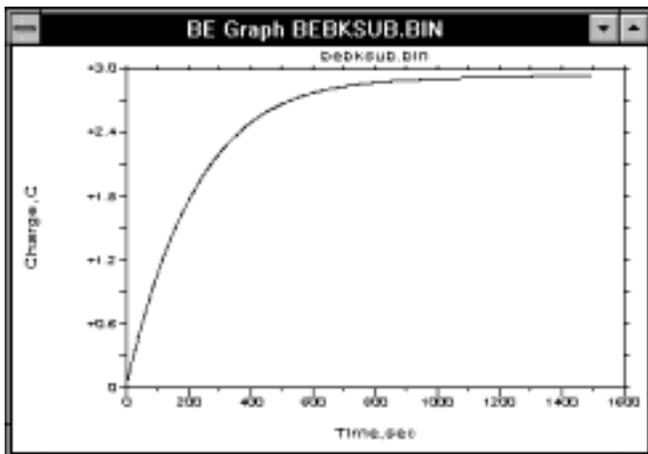
Figure 10-22. Typical charge vs. time plot for **BE**.
