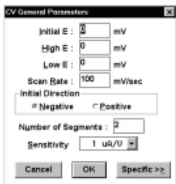
Figure 4-2. General Parameters dialog box for CV.
