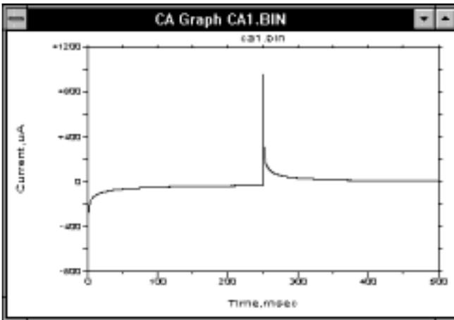
**Figure 10-6.** Chronoamperogram (current-time) response for double-potential-step CA.
