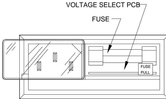
**Figure 2-1.** Power connector and voltage select.
