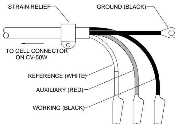
**Figure 2-2.** Cell (electrode) end of cell cable.
