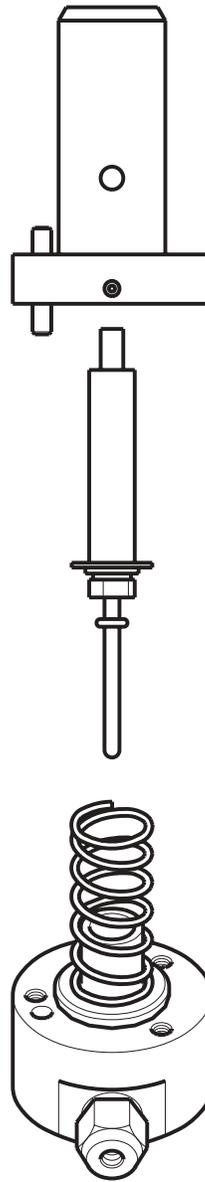
Figure 6.3. Exposing the plunger seal.
