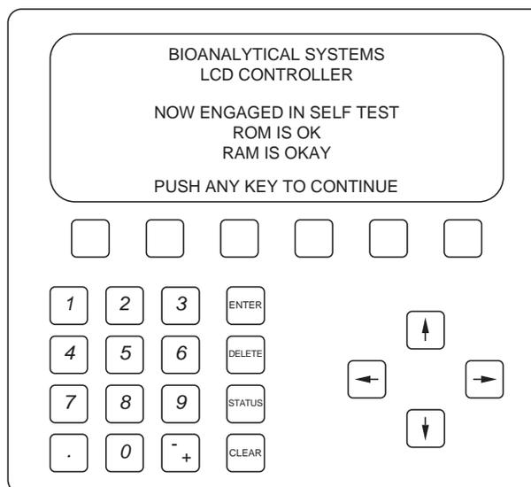
The row of blank buttons directly under the display become active when function labels appear in the display just above them.
