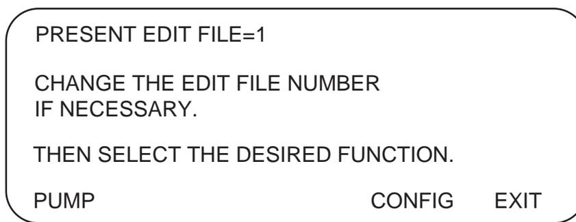
2. Press the key below the word PUMP, and the screen in Figure 5.5 will appear. This is the main programming screen for the pump.
