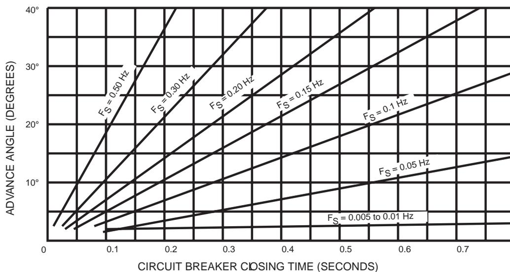
Figure 1 - Slip, advance angle, and breaker closing time
