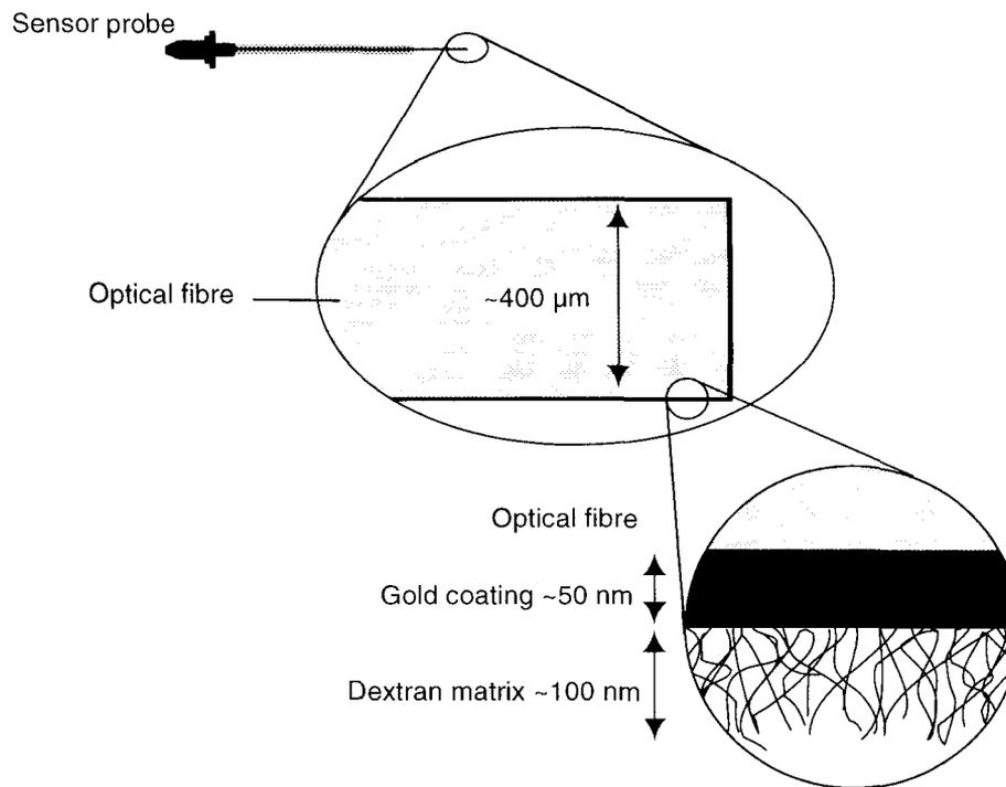
**Figure 2-2.** Structure of the tip of Sensor Probe CM5, showing the relationship between the optical fibre, the gold coating and the dextran matrix.
