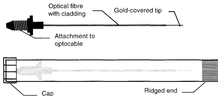
**Figure 2-1.** Construction of the sensor probe (top) and protective tube (bottom) with the position of the sensor probe marked in grey.
