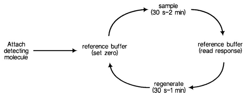
**Figure 4-1.** Analysis cycle using directly coupled detecting molecule.
