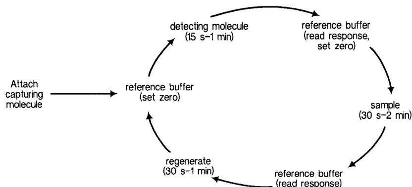
**Figure 4-2.** Analysis cycle using captured detecting molecule.
