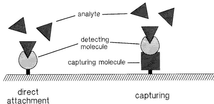
**Figure 3-1.** Two ways of functionalizing the sensor probe.
