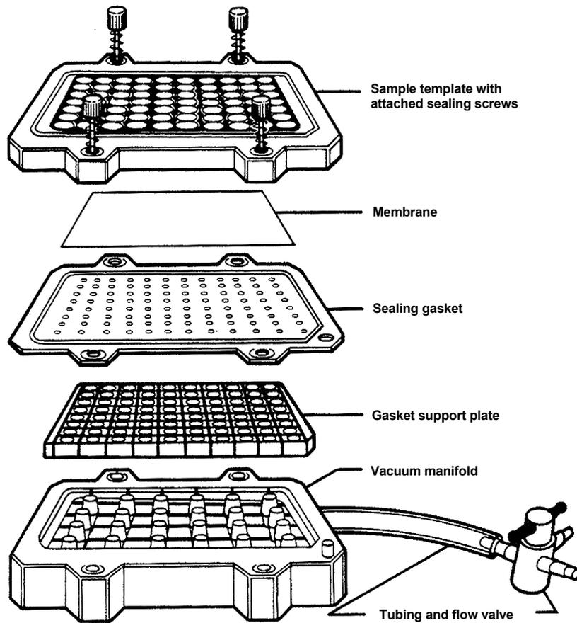
Fig. 1. Diagram of proper Bio-Dot apparatus assembly.
