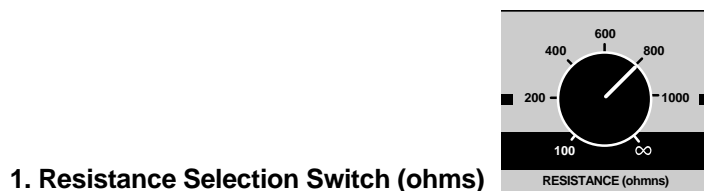
Fig. 3.2. The front control panel of the Pulse Controller II apparatus. Resistor selection switch (1) and shocking chamber output jack (2).
