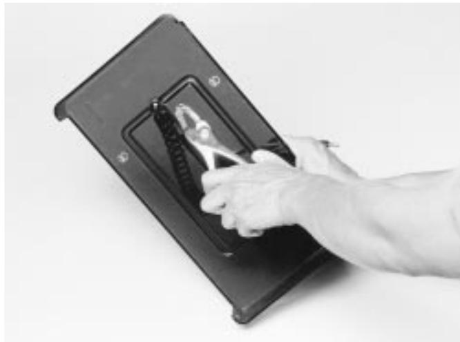
2. Locate the punch out tab in the upper right corner on both sides of the central cooling core.
