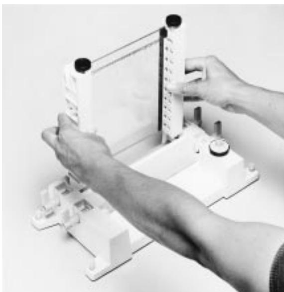
4. With the short glass plate facing the cooling core (and the locating decal on the clamps facing the core), position the gel sandwich so that the grooves in the upper portion of the clamps are fitted onto the locating pins on the central cooling core.\* The gel sandwich should be positioned at an angle of  $\leq 20^\circ$  with the cooling core. Keeping this angle to a minimum and lubricating the gasket will prevent distortion of the gasket while the sandwich slides into place.
