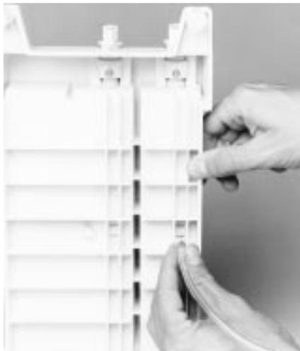
3. Stand the casting stand up on a level surface, add APS and TEMED to the monomer solutions, and begin pumping the gradient monomer solution.
