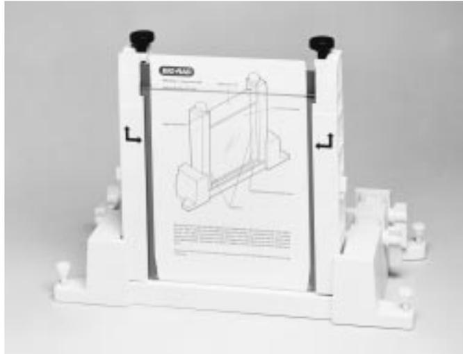
7. Simultaneously push inward on both clamps at the locating arrows, and tighten both clamp screws just enough to hold the sandwich in place. Pushing inward on both clamps at a point below the locating arrows will insure that the spacers and glass plates are flush against the sides of the clamps.
