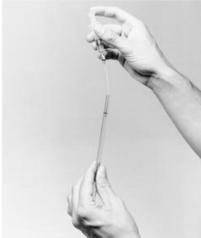
3. Attach a piece of silicone tubing to a 1 ml syringe and to the outside wall of the glass tubes on the top end of the tube. Using the syringe filled with distilled water, apply a firm, even pressure to start the gel extruding from the tubes. As the gel moves further out of the tube, apply less pressure so that rate of extrusion remains constant. Care must also be taken not to extrude too quickly. Only slight pressure is required to remove the last 1-2 cm of gel from the tube.
