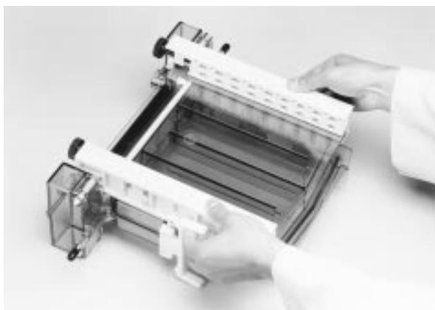
6. Turn the central cooling core to its other side, and repeat steps 1 through 5 to attach the second gel sandwich to it.
