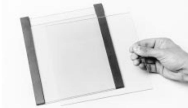
3. Apply the sandwich clamps as described in Section 3.1, steps 3-4. Insert two alignment cards between each of the sandwiches to keep the spacers upright during sandwich alignment. Align, and then cam the whole assembly into the casting stand. The sandwiches are now ready for gel casting.
