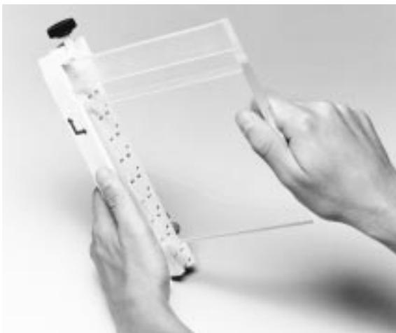
**Note:** Failure to slide the dam up completely to the top of the clamp will result in an upper buffer leak.
