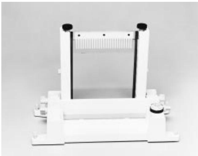
Generally, an overlay solution is not necessary for polymerization when a comb is in place.
