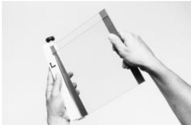
4. Place the right clamp on the right side of the plates, and tighten the clamp screw.
