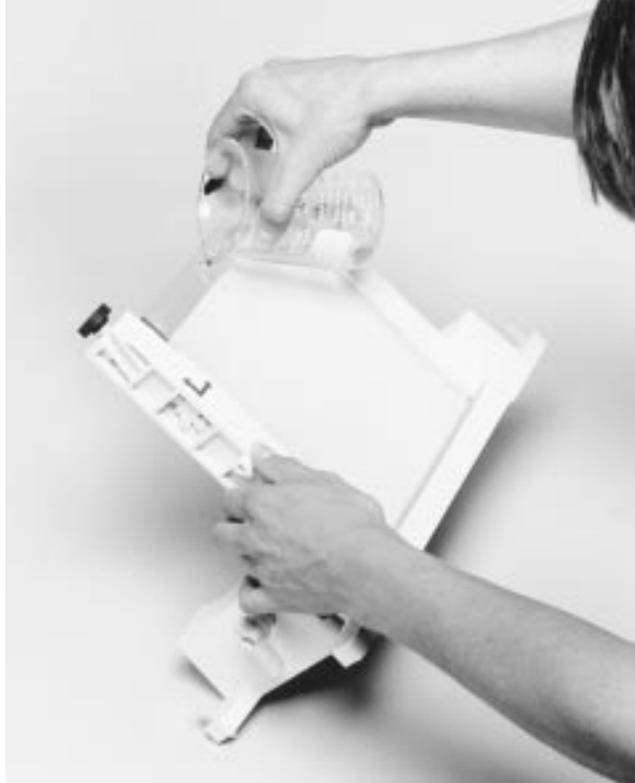
**Note:** If an incubator is not available, molten (75 to 85 °C) agarose can be poured into a room temperature sandwich assembly. This temperature is high enough to prevent premature gelling of the agarose, yet low enough to prevent cracking of the glass plates.
