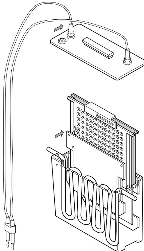
**The anode electrode is removed from the standard position and placed 4 cm apart from the cathode. The cable is also moved to line up with electrodes.**
