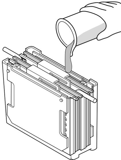
**Note:** For high intensity runs (4 cm inter-electrode distance) only one cassette can be placed in the tank. The Super Cooling Coil must be used. It is placed outside the electrodes. See Section 2.2, high intensity field option. Two cassettes can be run with the Super Cooling Coil in the standard field with the electrodes 8 cm apart, and three cassettes can be run at low voltage without the super cooling coil.
