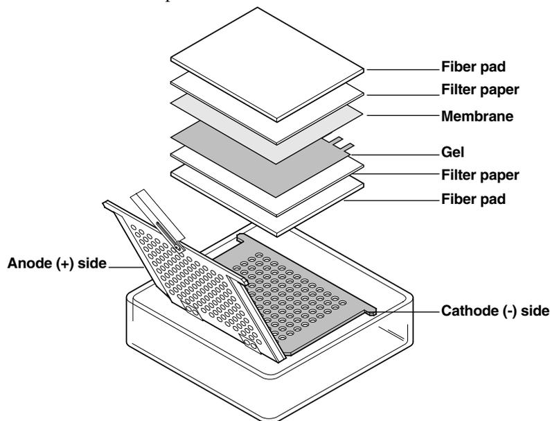
4. Close the cassette firmly, being careful not to move the gel and filter paper sandwich. Lock the cassette closed with the white latch.
