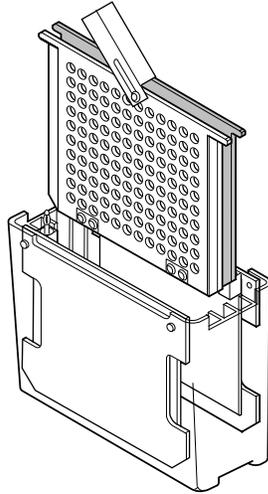
6. If running high intensity or high voltage with plate electrodes, add the super cooling coil in any available slot.
