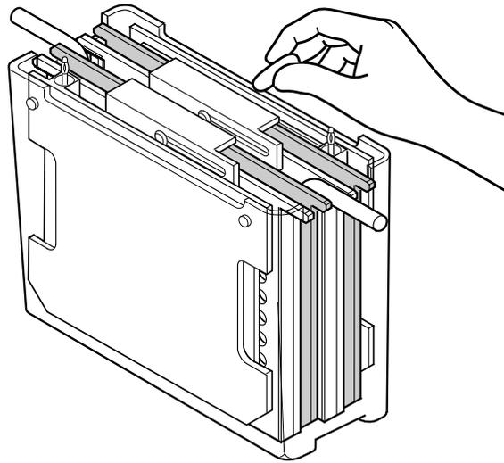
8. Put on the lid, plug the cables into the power supply, and run the blot. Refer to Section 3 for run times and voltage setting with various buffers.
