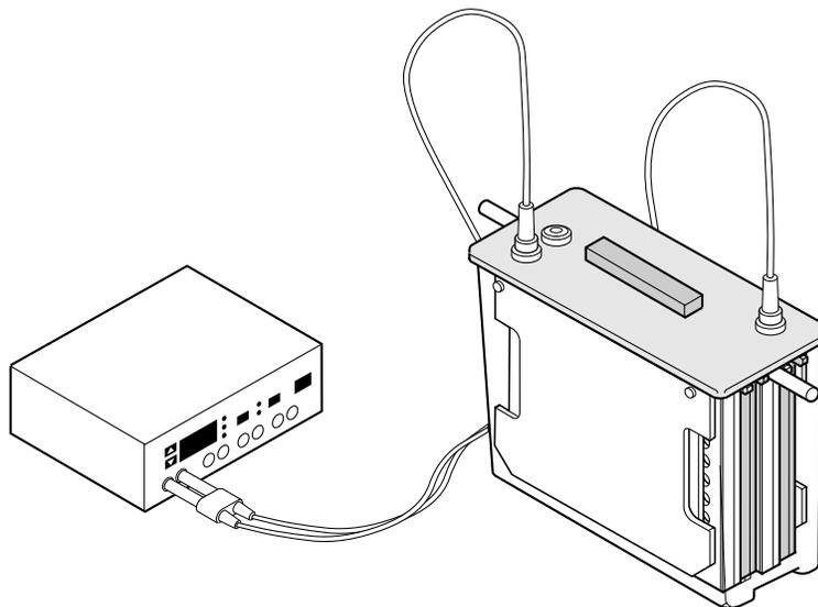
9. Upon completion of the run, disassemble the blotting sandwich and remove the membrane for development. Clean the cell, fiber pads, and cassettes with laboratory detergent and rinse well with deionized water.
