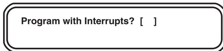
**Intrp =:** This prompt is asking if the program is to have interrupts (secondary pulses). Enter 0 if no interrupts are to be used and 1 if interrupts will be used. Interrupts are explained in Section 9.3.
