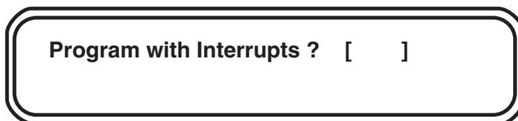
The display will ask if the interrupts will be 180° from the vector (i.e., go in the opposite direction the DNA is moving). If yes, enter 1. If you want to assign the angle of the interrupts, press 0 for no.
