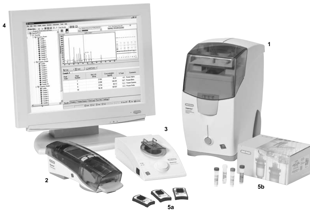
Figure 1.1. The Experion system includes the following components: (1) Automated electrophoresis station, (2) Priming station, (3) Vortex station for RNA analysis, (4) System operation and data analysis software, and (5) Analysis kits (sold separately), which include the (a) chips and (b) reagents for protein, standard sensitivity RNA, and high sensitivity RNA analysis.
