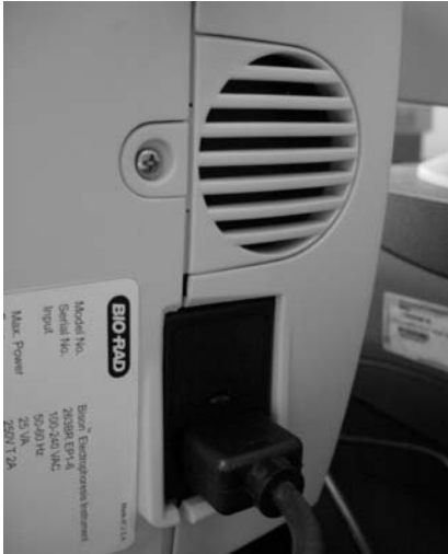
Figure. 1.5.2a. Power connection for electrophoresis station.
