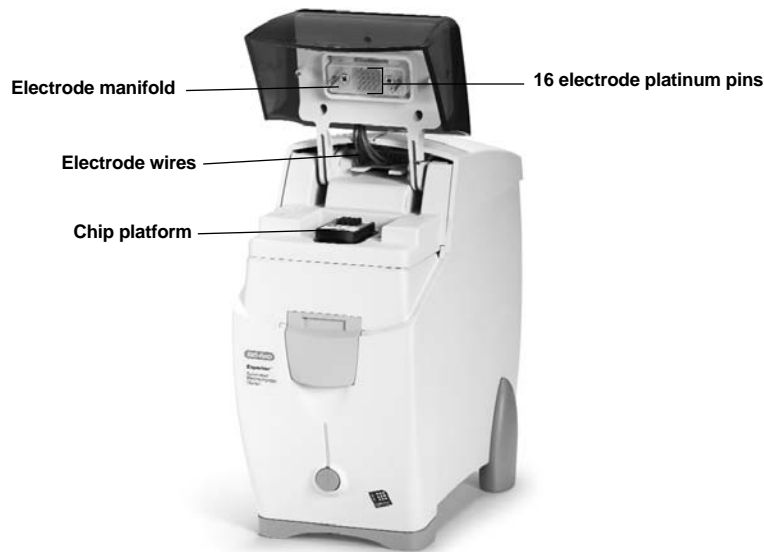
Figure. 1.3.1b. The Experion Electrophoresis station with lid open.
