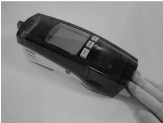
Figure. 2.4a. Opening the priming station.
