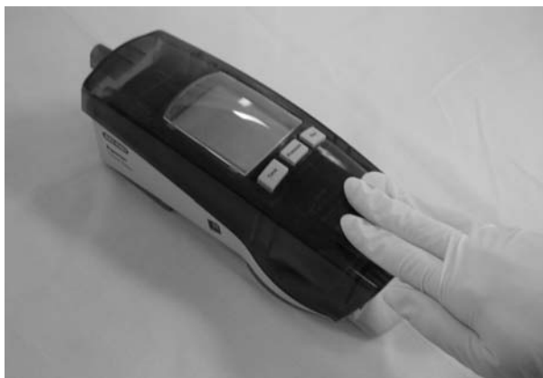
Figure 2.4d. Closing the priming station.
