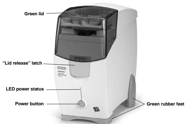
Figure. 1.3.1a. The Experion Automated Electrophoresis station.
