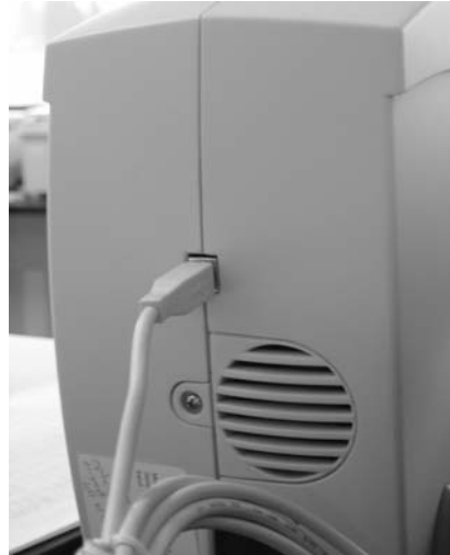
Figure. 1.5.2b. USB 2.0 cable connection for electrophoresis station.
