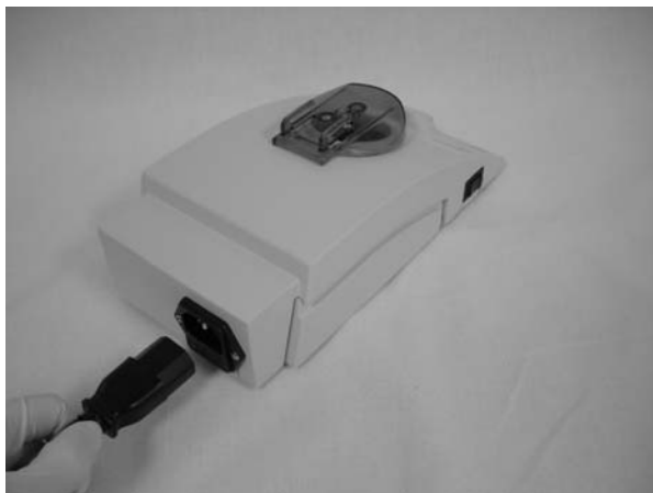
Figure. 1.5.2d. Power connection on the vortex station.
