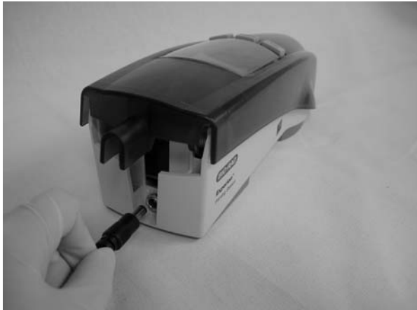
Figure. 1.5.2c. Power connection on the priming station.
