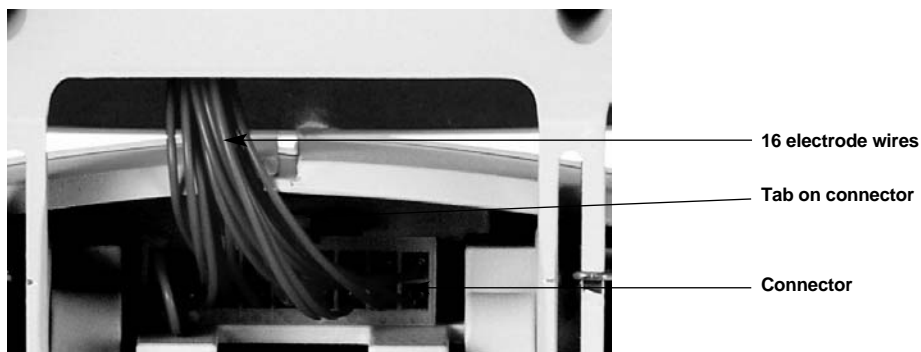
Figure 5.1b. Close up of the 16 electrode wires and connector.
