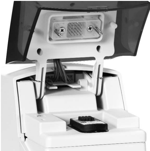
Figure. 2.6b. Proper chip placement in the electrophoresis station.
