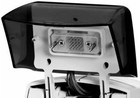
Figure 1a. Open electrophoresis station lid showing the electrode manifold.
