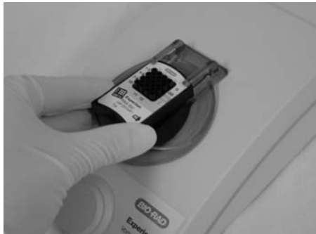
Figure. 2.5. Inserting a chip into the vortex station.
