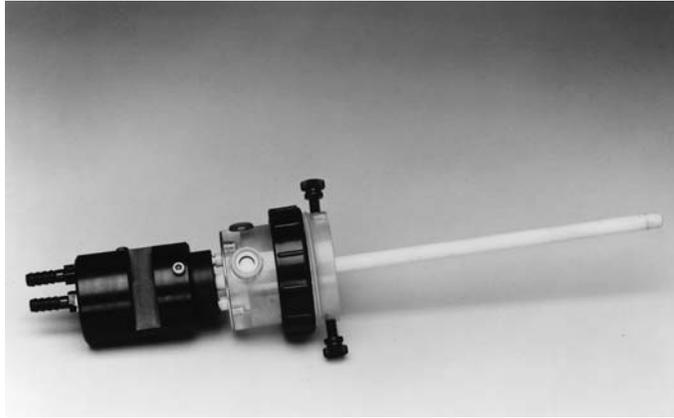
Fig. 3.3. Anode electrode assembled on the cooling finger.
