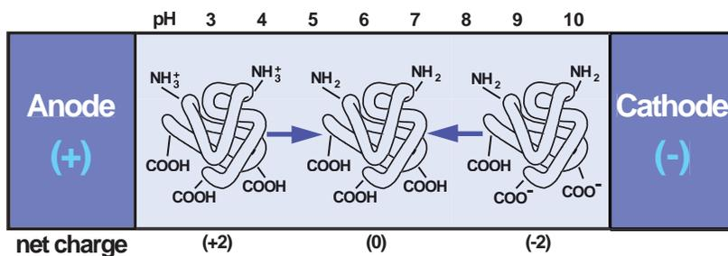
Fig. 1.1. Acidic Protein "Focusing" in a pH gradient.
