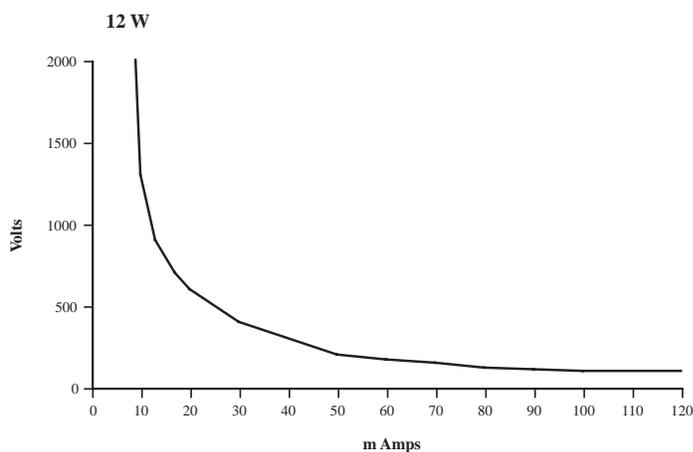
**Fig. 4.1. The maximum power that should be applied to the Rotofor cell is 12-15 W.** The graph shows the voltage and current readouts for setting a constant voltage power supply. If the current reading is too high at the set voltage (in the danger zone), reduce the voltage until a safe power level is obtained. **Watts = voltage x current.**
